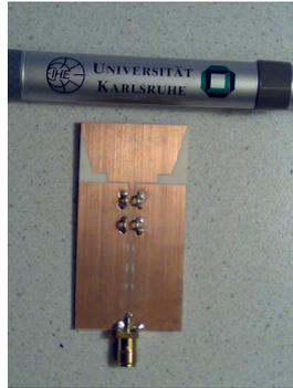
**Figure 4.2:** The fabricated antenna with the integrated bandpass filter.
