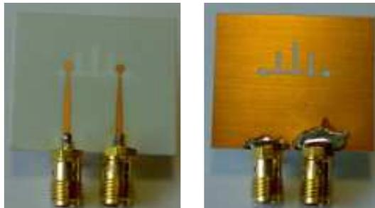
**Figure 3.20:** The fabricated filter with integrated lowpass-highpass sections: rear side (left) and front side (right).
