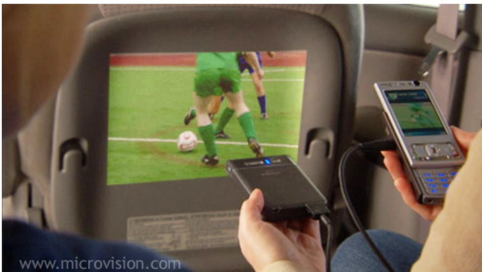
**Figure 3.4:** Prototype of an accessory pico-projector from Microvision, taken from [82].
