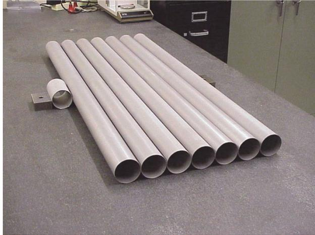
Figure 4: Thin walled beryllium tubes machined from bulk material
