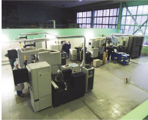
Fig. 3. Wire EDM machining area for beryllium tiles manufacturing
