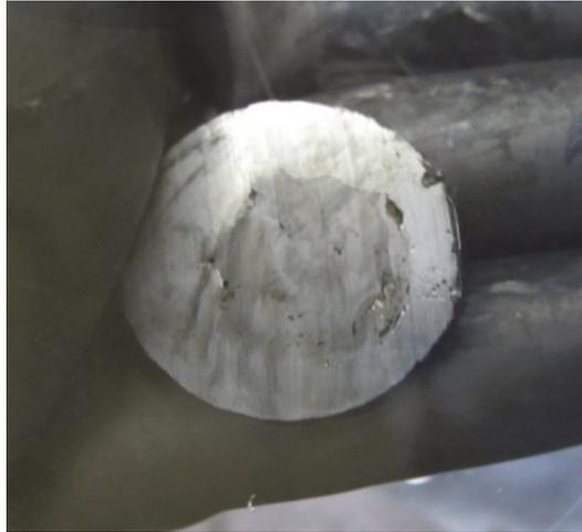
Fig. 3 Hot-extruded Be-Ti rod inside of a steel jacket
