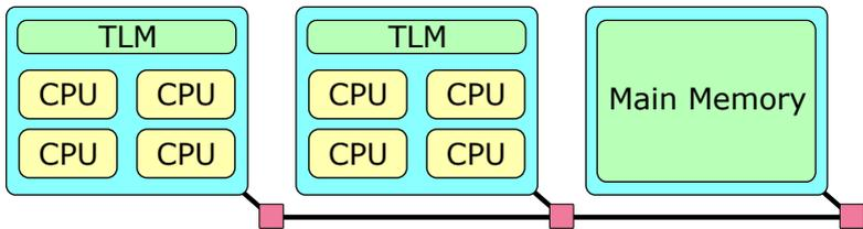
Figure 4.4: The hardware layout used for executing the resource-aware disparity map algorithm. A total number of 8 CPUs is distributed across two tiles containing additional Tile-Local Memory (TLM). Both compute tiles and a third tile containing the main memory are connected via a Network on Chip (NoC).
