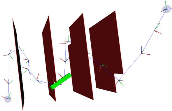
Figure 5.18: The test case *SerialWalls4* consists of four walls with opposing holes. The goal is to move the green beam from  $\rho_{start}$  on the left side of the walls to  $\rho_{goal}$  on the right side of the walls. *Source:* [Kröhnert et al., 2016] ©2016 IEEE
