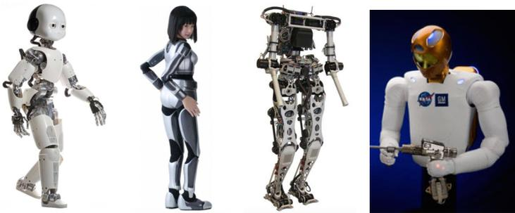
Figure 2.2: The humanoid robots iCub, HRP-4C, LOLA, and Robonaut 2. Sources: [Roncone et al., 2014] ©2014 IEEE, [Kaneko et al., 2009] ©2009 IEEE, [Lohmeier et al., 2009] ©2009 IEEE, [Diftler et al., 2011] ©2011 IEEE
