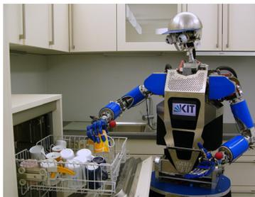
Figure 1.1: The humanoid robot ARMAR-IIIa while loading a dishwasher.
