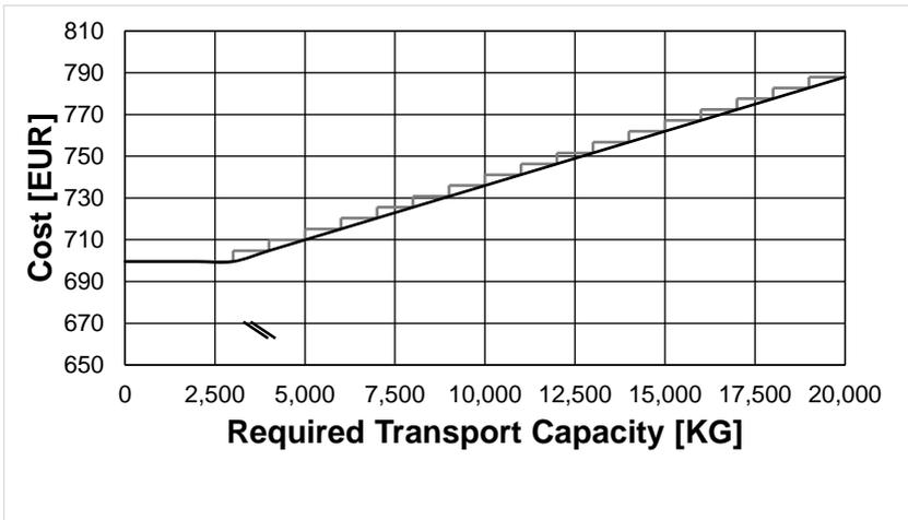
Figure 6.3: Costs of transportation as a function of shipment size.
