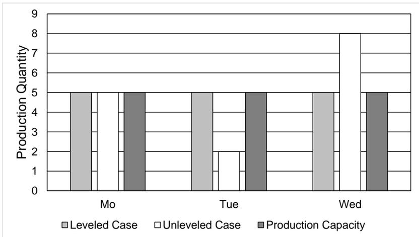
Figure 2.5: The idea of make-to-order leveling
