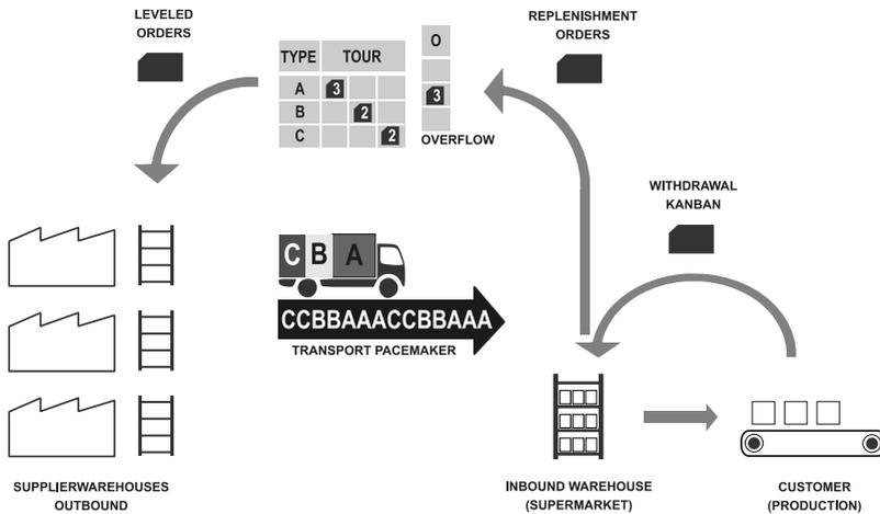
Figure 4.3: Heijunka leveled kanban system in materials supply
