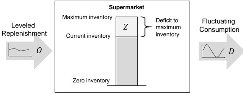
Figure 4.4: Description of the system state by the deficit to the maximum inventory
