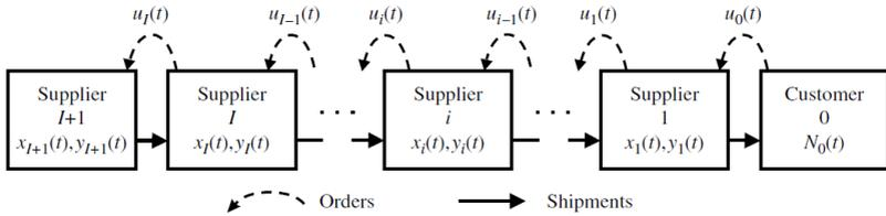
Figure 2.3: Supply chain model of Ouyang and Daganzo (2006)
