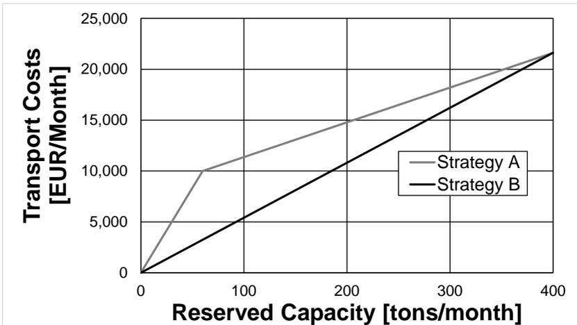
Figure 6.5: Transport costs per month as a function of the chargeable capacity  $\widetilde{TC}$  for strategies A and B
