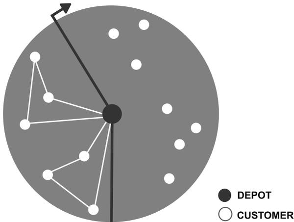
Figure 4.12: The sweep algorithm
