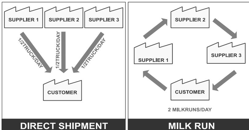
Figure 3.5: The idea of the supplier milk run
