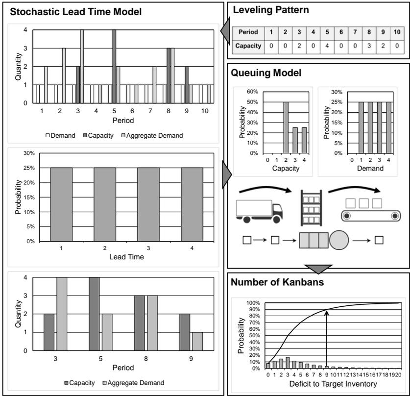
Figure 4.14: Interfaces between optimization model and inventory model
