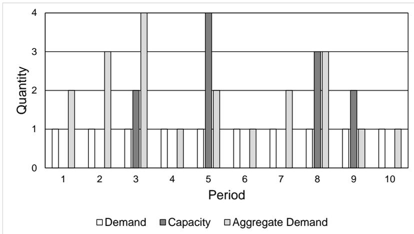
Figure 4.7: Leveling pattern with variable interarrival time
