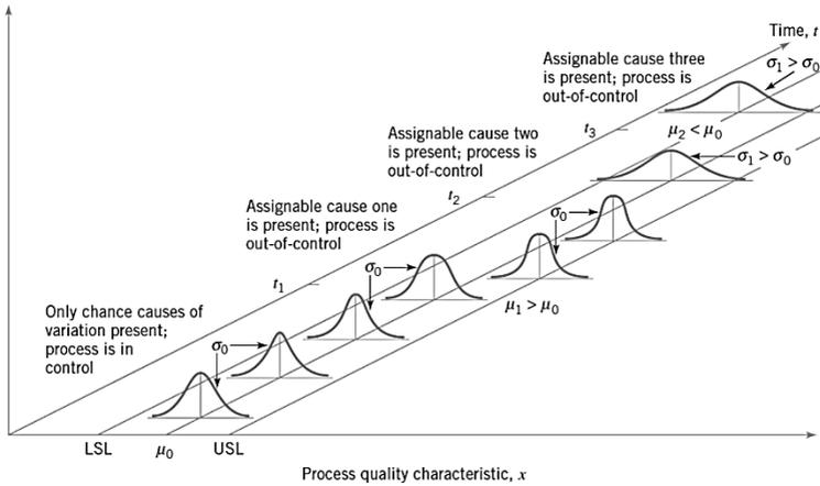
Figure 2.4: Chance and assignable causes of variation (Montgomery 2009)
