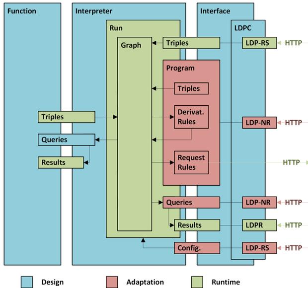
Figure 3.9: Smart Component – Architecture: Separation of Lifecycles
