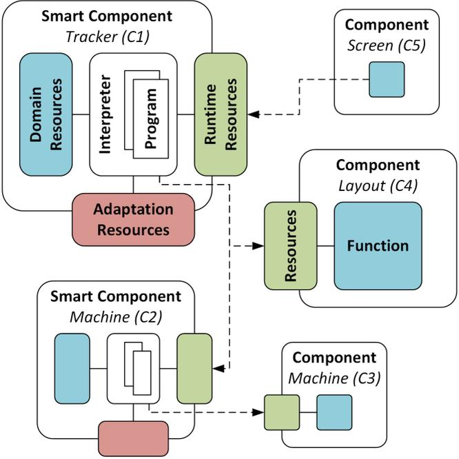
Figure 3.4: Smart Component-based Integration Architecture
