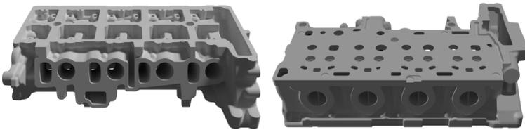
Figure 1.5: Cylinder head CAD model from two viewpoints.
