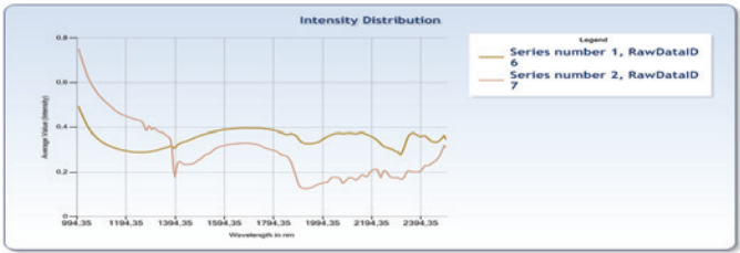
Figure 19.3: Intensity distribution for two different materials in the NIR and SWIR spectrum.
