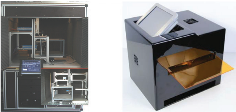
Figure 25.1: On the left is shown the materialscanner with the xvz-motors. SAMMI is shown on the right.
