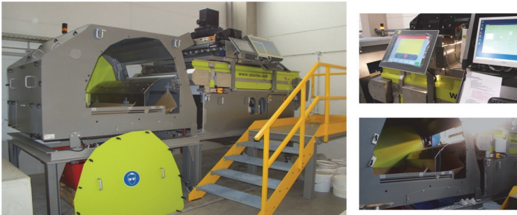
Figure 15.10: Near-infrared sensor based sorting machine for CDW
