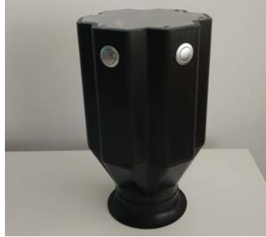
(b) PhasmaFOOD portable multi-sensor device
