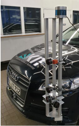
(a) Sensor setup prototype for UNICARagil project.
