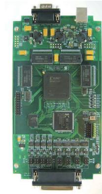
Abbildung 2.21: Spartan-3 FPGA Gateway Board
